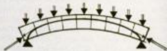
Compression structure alone: a masonry arch wedged into position along line of compression in a reversed catenary curve
